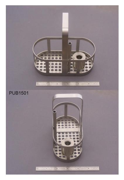
The **Small Basket** holds a **Sentry** and a test container up to 2.6" (66mm) in diameter. The entire assembly is inserted in a pasteurizer to run a test.
